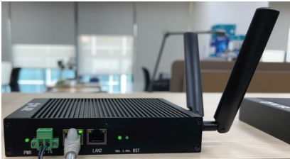
Figure 9.2 Connecting an Ethernet cable to the GW66.
