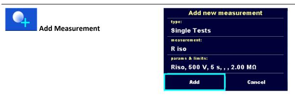
Figure 5.10: Add a new measurement menu
