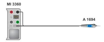
Figure 9.3: Connecting Tip Commander (A 1694)
