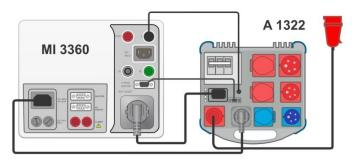
Figure 9.1: Connecting Active 3 Phase Adapter /plus (A 1322 / A 1422)
