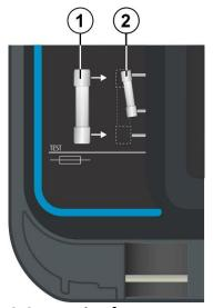
Figure 4.2:Connecting fuses to Fuse checker
