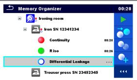
Figure 5.4: Example of status Measurements not completed with fail
