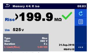
Figure 6.6: Single test memory screen
