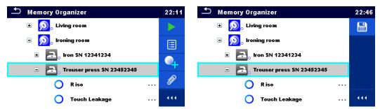
Figure 5.7: A structure object is selected in the tree menu
