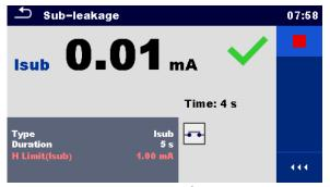
Figure 6.4: Single test screen (during measurement)
