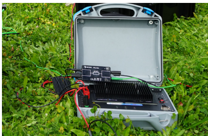
Body resistance simulation with 1 kOhm adapter A1597 for correct Touch Voltage calculation.
