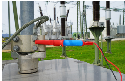
Kelvin Crocodiles ensure robust 4-wire connection for reliable results.
