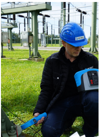
Flex or iron Clamps measures selective current from riser to grid.
